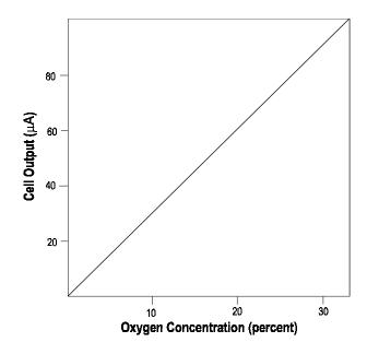
Figure 2-2. Characteristic Input/Output Curve for a Micro-Fuel Cell
